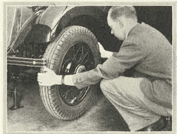
Looseness in track-rod joints will be betrayed by rocking the wheel round the steering swivel
