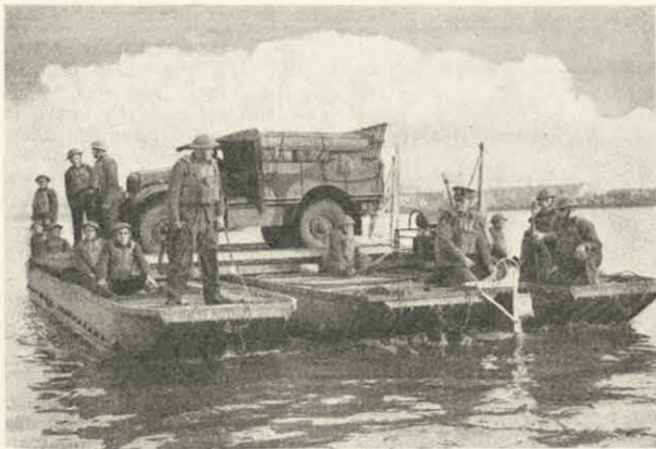
ROYAL ENGINEERS AT WORK — A pontoon raft coming ashore after ferrying a mechanised transport unit across a river, and (right) method of loading lorries aboard a tracked raft for ferrying
