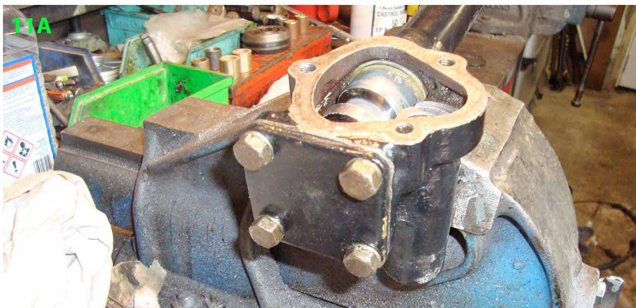
Picture 11: Shows the above shimming, and double checking each shim with a micrometer.
