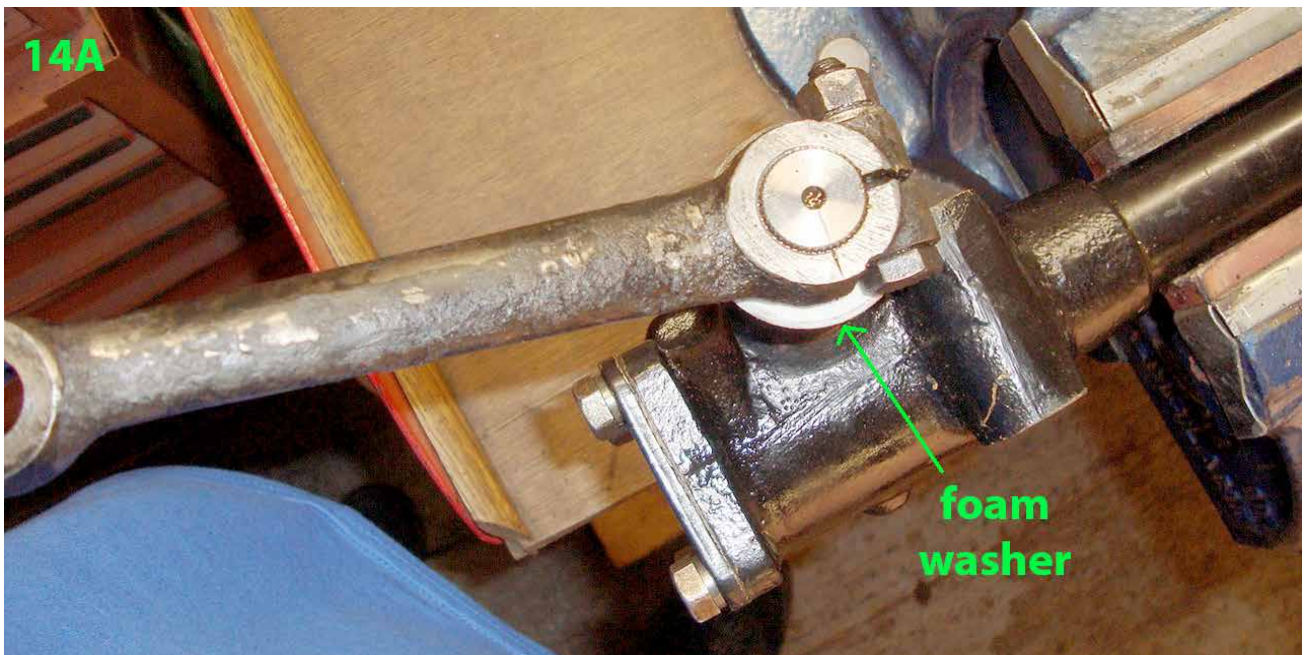
Picture 14: Aligning to markings and fitting the drop arm.
